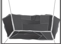
2) Apply thinset to PolyBench. Apply the thinset using a skim coat to all sides that will make contact with the walls and shower base.
