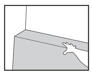
**4.** Level PolyBench by using a 2' level and placing it from the back wall running to the front edge. Also, level from left to right sides across the front. The "Top" side of PolyBench is pre-sloped with a ¼" per foot running slope. If a steeper slope is desired, remove PolyBench and apply more thinset to the back lower corner (plastic shims can be used as well if desired). Once done, repeat steps 3 & 4.
