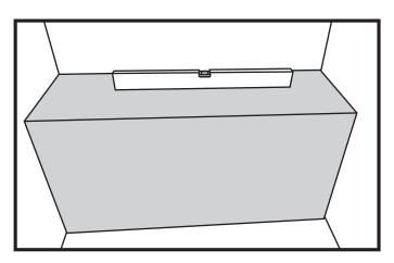
**5.** Remove any debris and ensure PolyBench and wallboard are clean. Apply drywall mesh tape over all seams where PolyBench meets the wallboard. Secure mesh tape in place by pressing it in place with a trowel.
