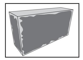
3. Install PolyBench in the desired location, first by placing the bottom front edge on the pencil line. Slowly set the back side down until PolyBench makes full contact with all sides to the walls and shower base. Apply pressure by pressing down and back on PolyBench to ensure a secure fit.
