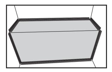
6. Apply a skim coat of Polymer Modified Thinset over the mesh tape to secure the joint between PolyBench, and the wallboard. Flash out thinset if nessecary. Once the thinset is cured, a coat of waterproof membrane may be rolled or brush on.
