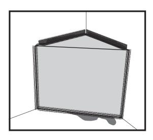
**6.** Apply a skim coat of Polymer Modified Thinset over the mesh tape to secure the joint between PolySeat, and the wallboard. Flash out thinset if nessecary. Once the thinset is cured, a coat of waterproof membrane may be rolled or brush on.
