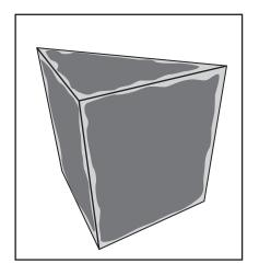
2) Apply thinset to PolyBench. Apply the thinset using a skim coat to all sides that will make contact with the walls and shower base.
