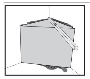
**4.** Level PolySeat by using a 2' level and placing it from the back corner running to the front edge. Also, level from left to right sides across the front. The "Top" side of PolySeat is pre-sloped with a ½" per foot running slope. If a more steep slope is desired, remove PolySeat and apply more thinset to the back lower corner (plastic shims can be used as well if desired). Once done, repeat steps 3 & 4.
